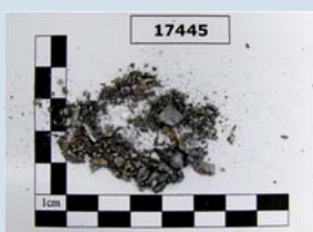
Impact of 2 mm Al_2O_3 ceramic body positioned in front of backing A: armor glass backing B: Al alloy (opaque armor)
